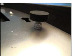
**Step 4:** Place the seat on the frame and evenly adjust the height of the four rubber buffers (middle and back) so the seat does not touch the frame
