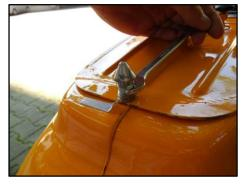
Step 3: Remove the cone bolt for the locking mechanism of the old seat.
