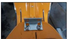
**Step 8:** Mount the locking bracket to the front of the frame together with the two M7x20 hexagon bolts and M7 washers as shown on the photo to the left.
