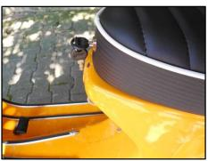
**Step 6:** Put the seat on the bolts and push it backwards. Next, pull up the seat in the front and back to determine the vertical clearance. Reduce the clearance to a minimum by adjusting the height of the bolts accordingly. Tighten the counter-nuts afterwards.
