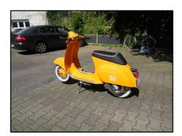
**Step 9:** Position the seat on the mounting system right before the locking bracket and slide it backward. Turn and remove the key. If too much horizontal clearance of the seat is detectable, adjust the clearance be repositioning the locking bracket on the frame. Removal: Unlock the seat and move it forward by pushing against the back.
