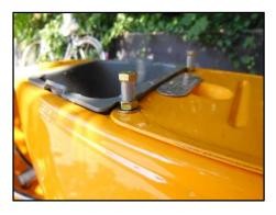
**Step 5:** Screw in the three M7x55 pan-head allen bolts in the front and back of the tank together with the M7 washers and nuts. Tighten the counter-nuts slightly.
